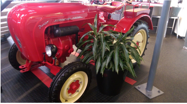
Porsche Diesel Junior, circa 1952-63, 14 hp, 822 cc, single cylinder, air cooled
